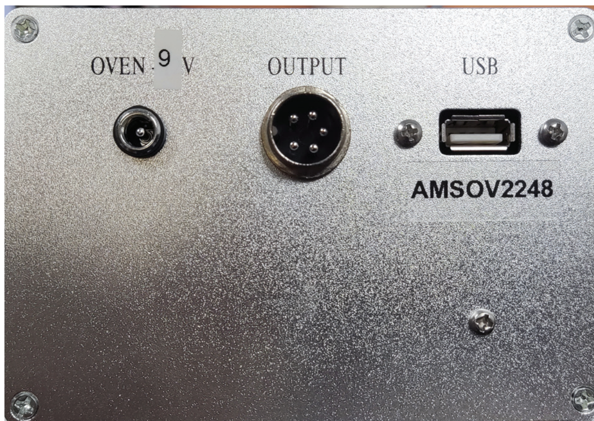
FIGURE 3. Oven controller (temperature controller) back panel
