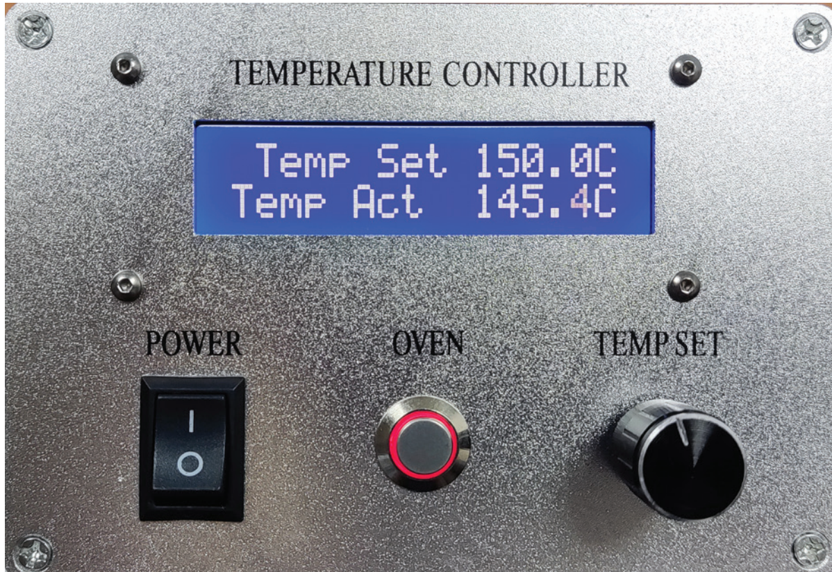
FIGURE 2. Oven Controller (temperature controller) front panel
