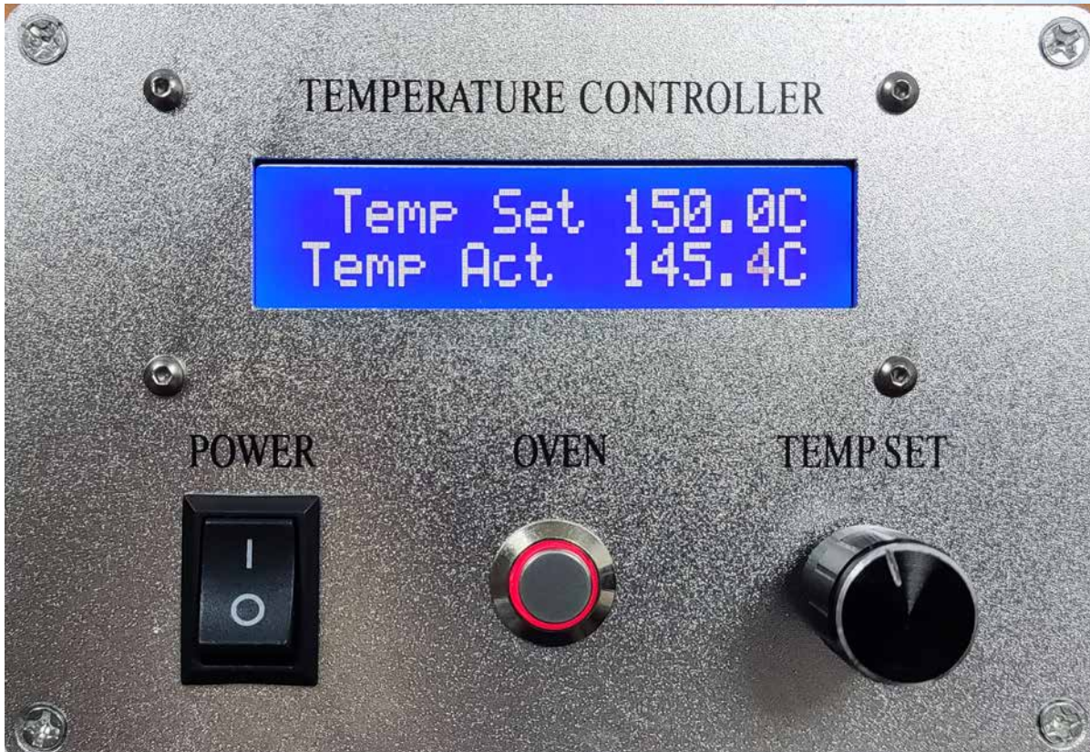
FIGURE 2. Oven Controller (temperature controller) front panel
