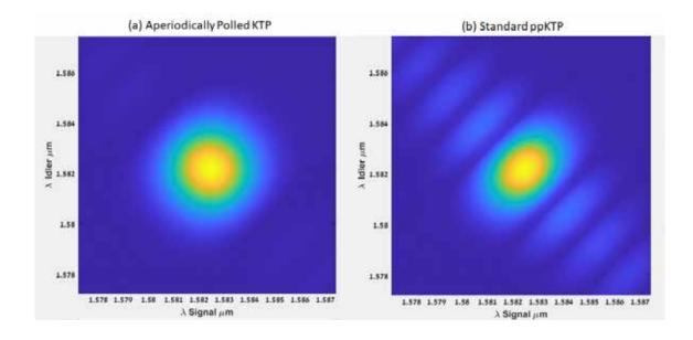
Raicol's High Purity APKTP is a uniquely designed KTP crystal that maximizes spectral purity at telecom wavelengths. It is a type-2 crystal, suitable for pumping with Ti-Sapphire lasers (775-795nm) with a degenerate SPDC output. Using the HP APKTP enables quantum researchers to achieve higher spectral purity without any external narrowband filters, therefore reducing the losses in the system and increasing the quantum properties of the entangled state.
