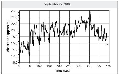
Time dependent dynamics of absorption in the crystal bulk @532 nm under self-radiation of 532nm. This parameter indicates the effectiveness and gray tracking resistance of the crystals. This is correlated to the crystal's lifetime - the lower the value, the longer the expected lifetime.
